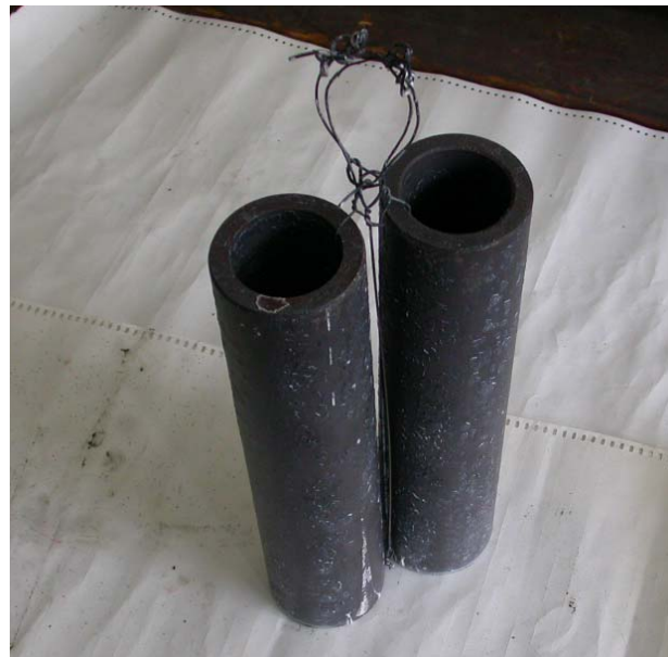
Figure 1. Position of pieces during the heat treatment
