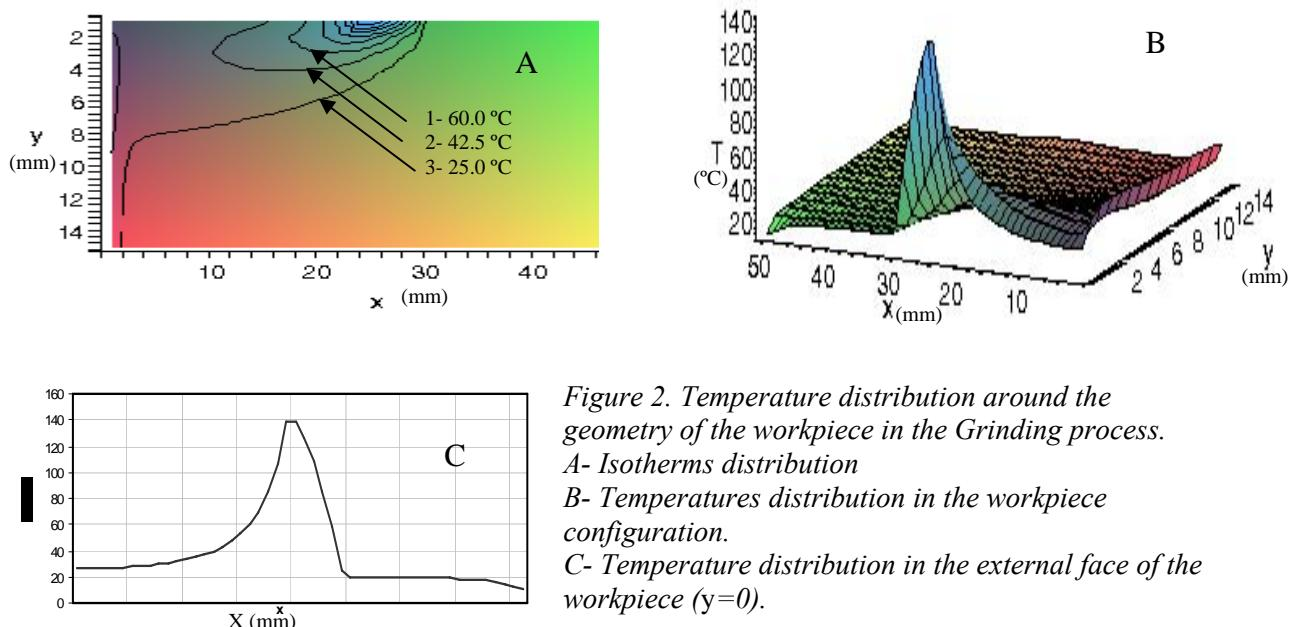
*Figure 2. Temperature distribution around the geometry of the workpiece in the Grinding process.*
