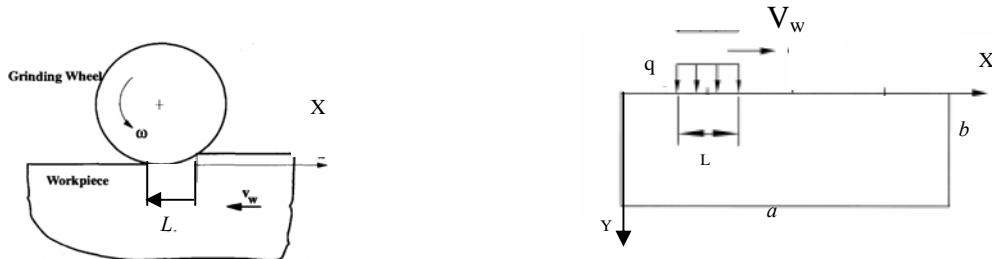
Figure 1a. Schematic diagram of a Grinding process.
