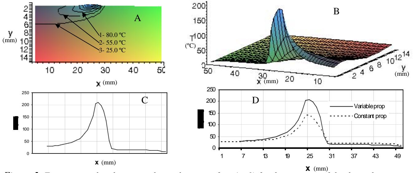
Figure 5. Temperature distribution on the workpiece surface ( $y=0$ ) for the variation of the thermal conductivity due to the variation of the temperature.
