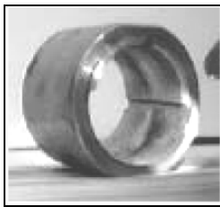
Figure 4. Bimetallic steel-bronze bush.
