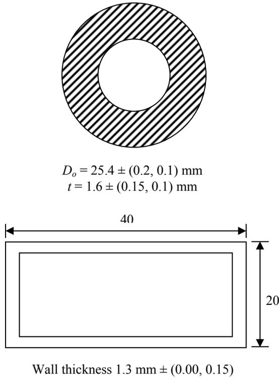
Figure 1. Profile sections of tube and box dies used in the study
