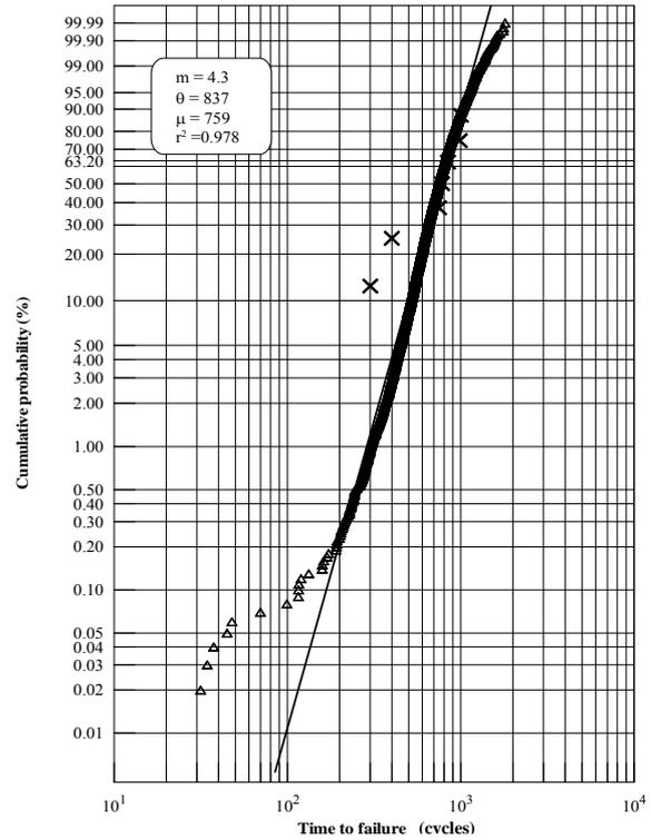
Figure 2. Weibull model of the simulated fracture-failure data
