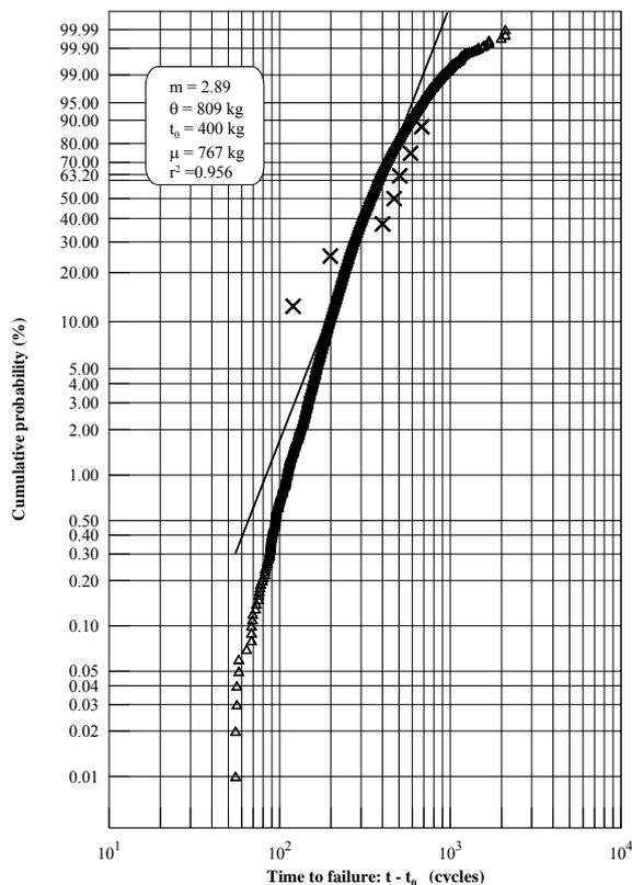
Figure 3. Simulated wear failure data and 3-parameter Weibull fit
