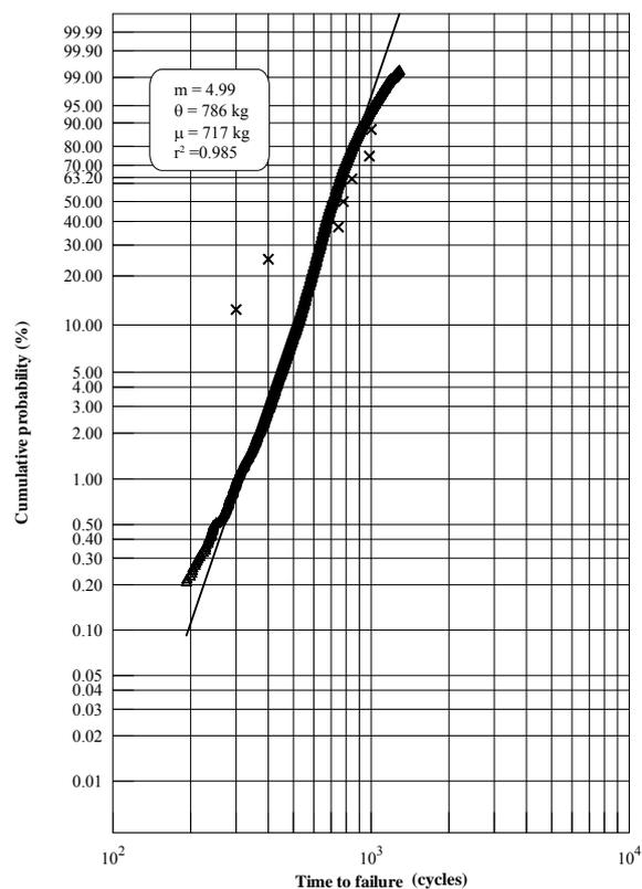
Figure 4. Weibull plot for simulated competing fracture-wear data
