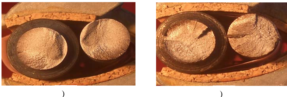
Figure 3 Fatigue fractured surfaces: (a) tempered at 400°C for 30 minutes; smooth surface, (b) tempered at 200°C for 30 minutes; rough surface
