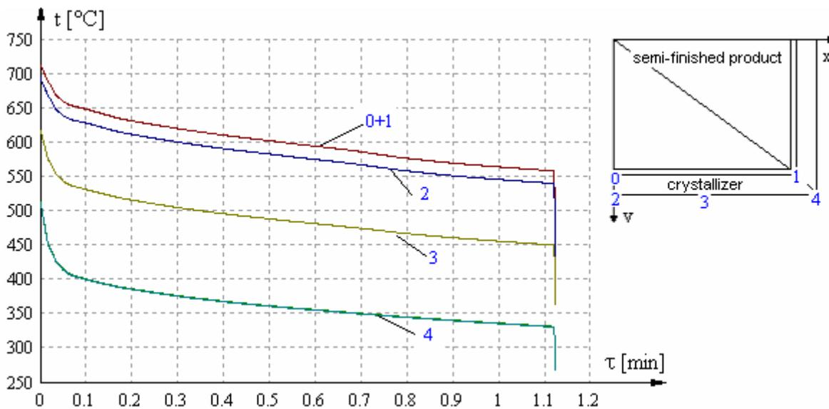
Figure 5. Temperature variation in the crystallizer, function of time
