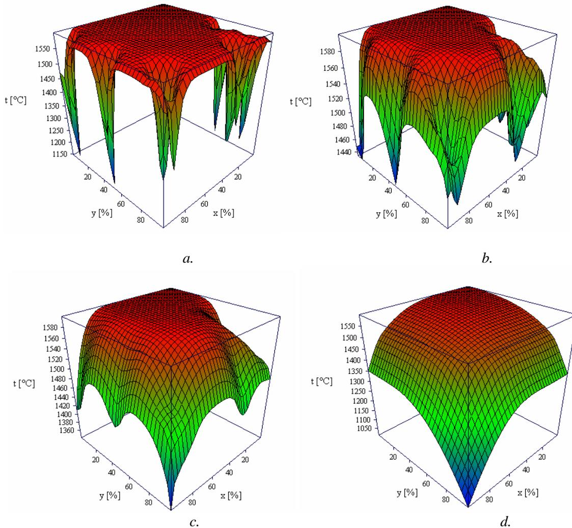
Figure 6. Temperature distribution in the continuous cast blank: at 3s (a), 10s (b), 30s (c) since the micro-coolers adding in the secondary cooling zone (d).
