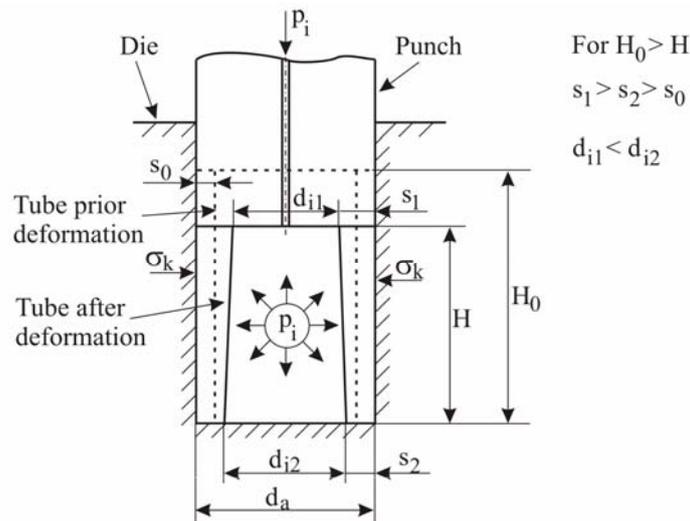
Figure 3. Upsetting of tube under inner pressure
