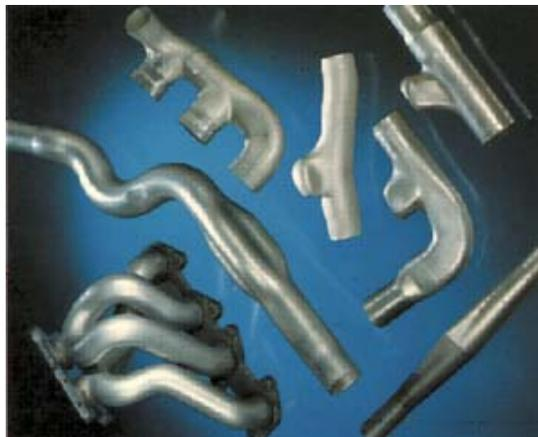
Figure 1. Components manufactured by THF
