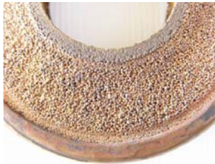
Fig. 7. Assembling of bronze filters in copper case
