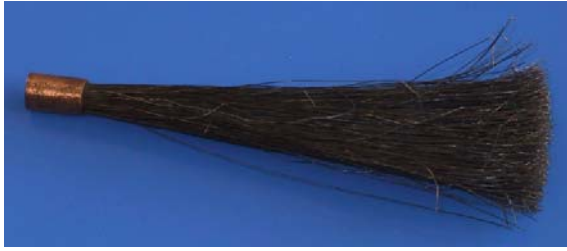
Fig. 5. Part with unidirectional steel fibers in copper holder ( d = 0.7 \text{ mm} )
