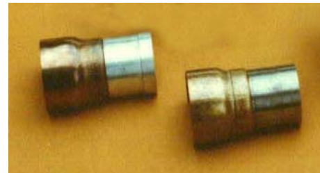
Fig. 8. Welds of the pipes (copper-steel, copper-titanium)
