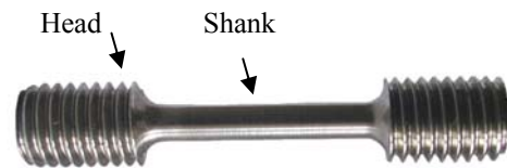
Figure 1. Creep test sample, \phi 5 mm, length 25 mm
