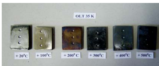
Image 1. Set of test rods made of OLT 35K, unused material, tried at high temperatures
