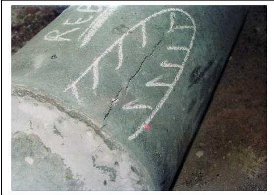
*Figure 1. The mill rolls no. 0950/03736, which presents longitudinal crack (the rejected roll registered at casting).*
