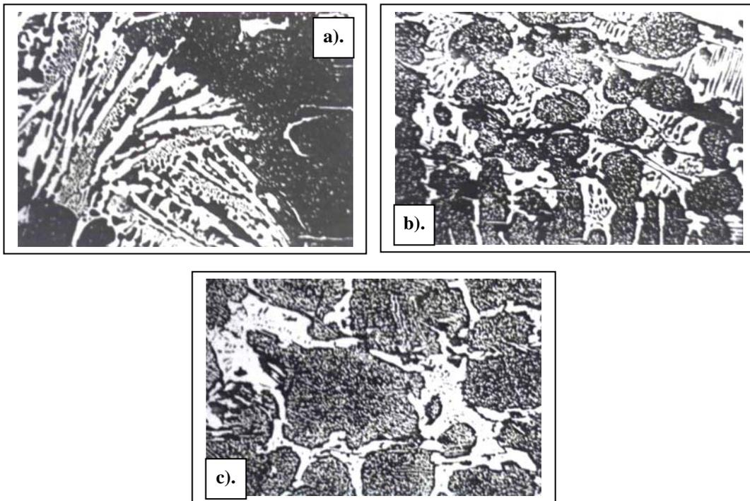
Figure 5. The microstructure of the roll 0470/02900 rejected because of the "tough" spots (growth: 100:1 - attack: nital 2%): a, b - zone with tough spots (425 HB); c - normal zone, without defects (360HB).
