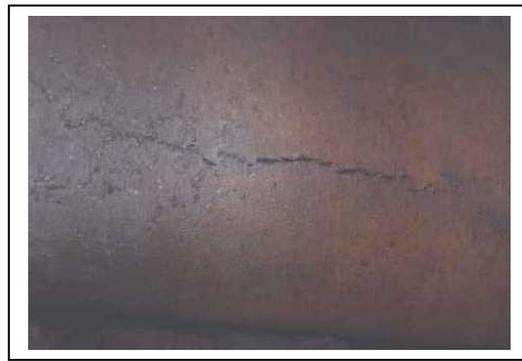
*Figure 2. The mill rolls no. 0963/03745, which presents longitudinal crack.*
