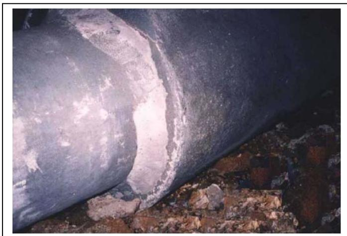
*Figure 3. Casted roll presenting adherence (in the zone between inferior neck and table).*
