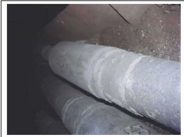
Figure 4. Casted roll presenting adherence (in the zone of the superior neck).
