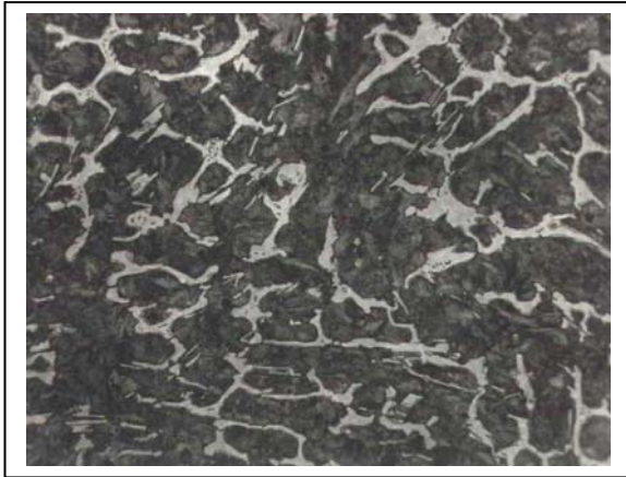
Figure.3. Microstructure of the roll's face (in casted state), nital attack 2%, growth 100:1.
