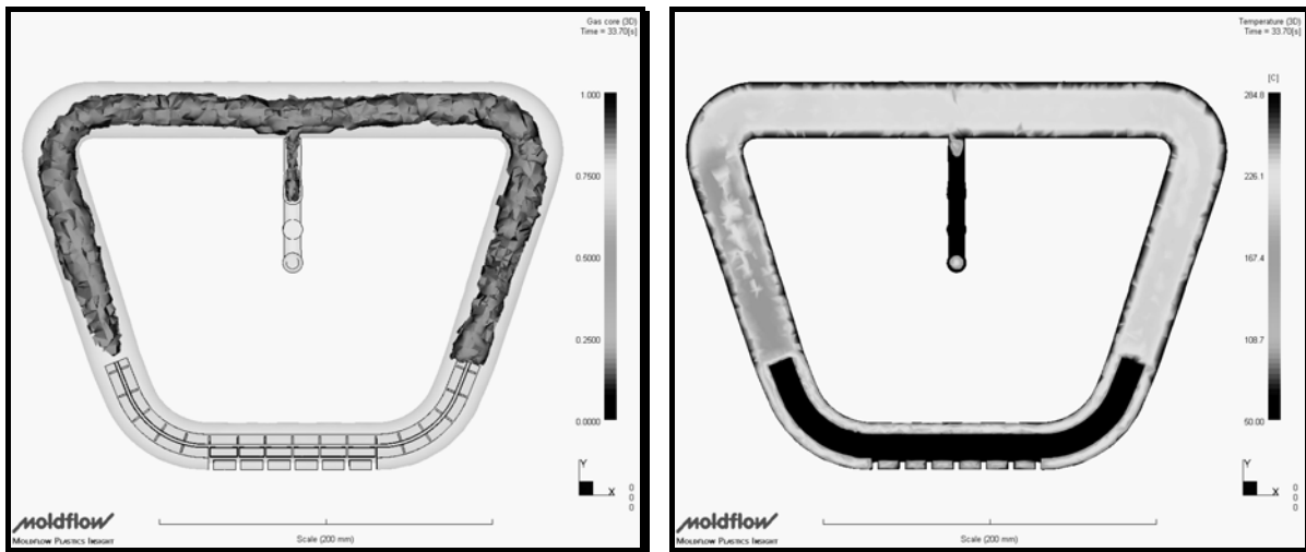
Figure 4: Cavity made by gas in 33 rd second of the injection cycle and temperature field in the part
