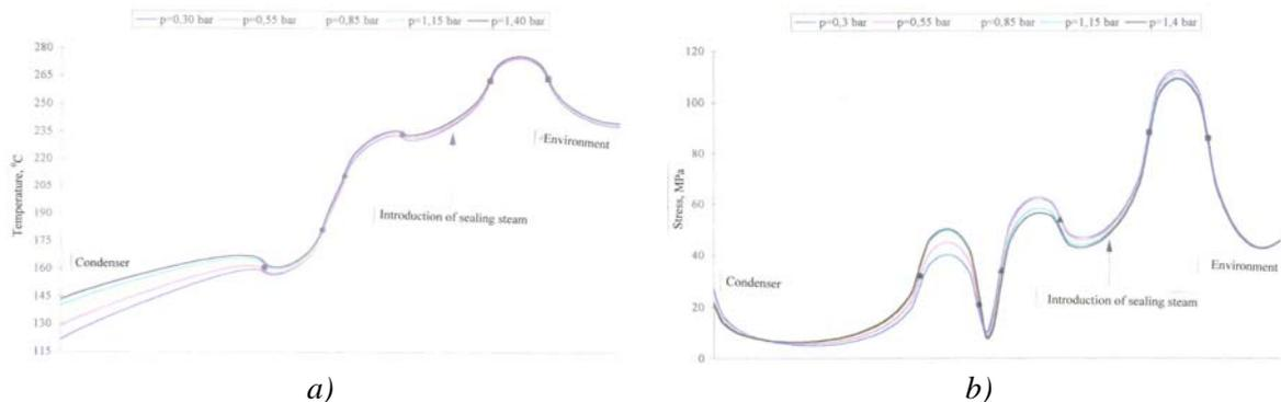
Figure 3. The distributions of temperatures (a) and equivalent von Mises stresses (b) along the region of the rear-end labyrinth gland
