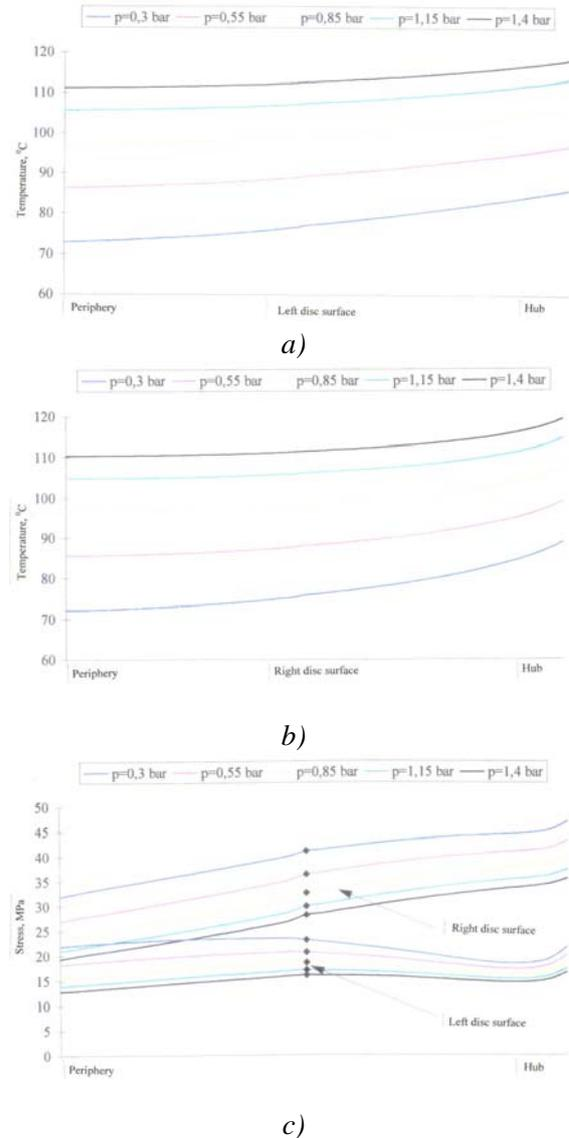
Figure 2. The distributions of temperatures on left (a) and right disc surface (b) of last turbine stage, and the distributions of equivalent von Mises stresses for both disc surfaces (c)
