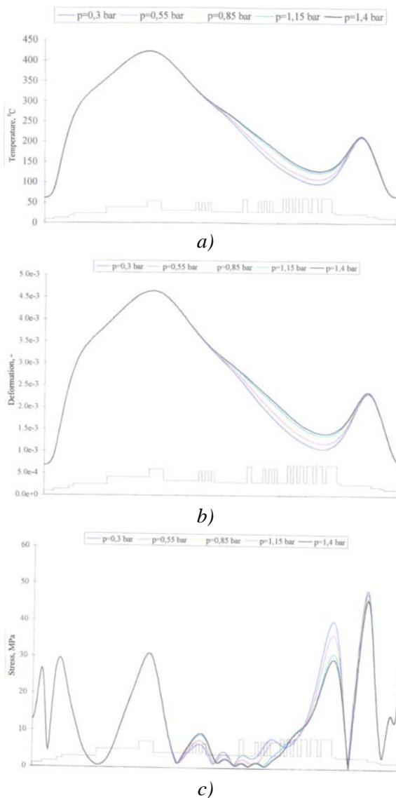
Figure 1. The distributions of temperatures (a), thermal deformations (b) and equivalent von Mises stresses (c) along the rotor central bore
