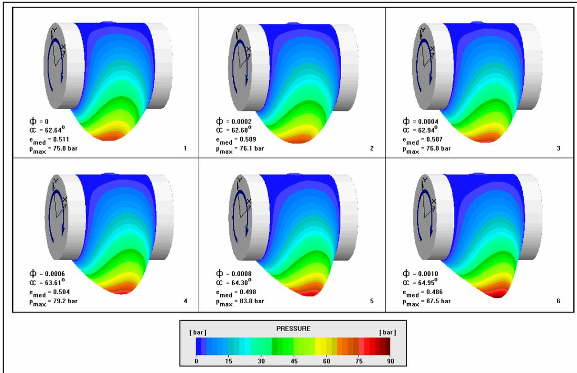
**Bearing sizes:** diameter,  $D = 100 \text{ mm}$ ; length,  $L = 80 \text{ mm}$ ; radial play,  $J = 0,2 \text{ mm}$ .
