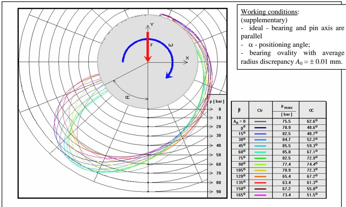
Figure 2. Hydrodynamics pressure distribution in bearing median plane (“oval” form of interior surface)
