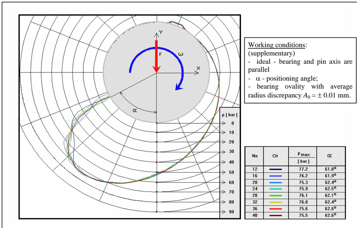
Figure 3. Hydrodynamics pressure distribution in bearing median plane (rippled form of interior surface)
