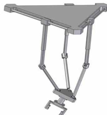
Figure 2. The CAD model of the 3-PPRS mini-manipulator
