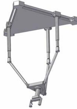
Figure 4. The CAD model of the 3-PPSR mini-manipulator
