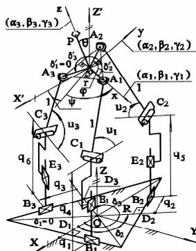
Figure 1. Kinematic scheme of the 3-PPRS mini-manipulator
