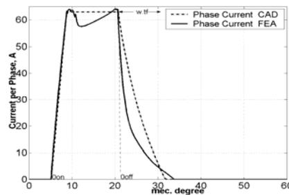
Figure 5. Evaluation of CAD and FEA phase-currents outputs for the designed
