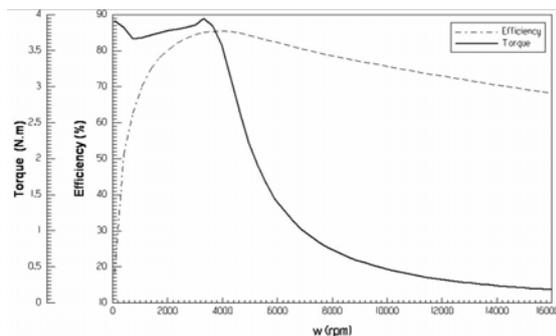
Figure 7. SRM Torque-Efficiency vs. Speed by FEA
