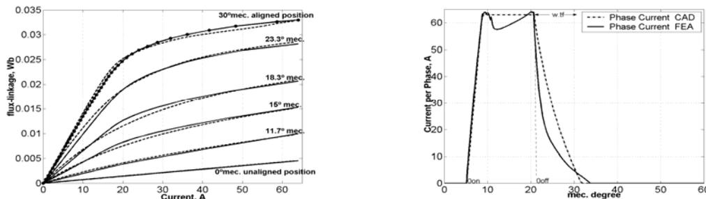
Figure 4. Comparison of the analytical CAD flux linkage curves and FEA flux result.
