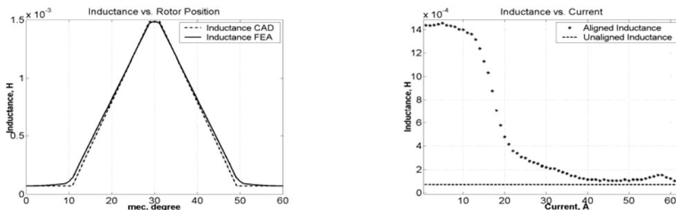
Figure 3. a) Comparison of aligned-unaligned CAD and FEA inductances versus rotor positions with current  $\leq I_{sat}$  b) Aligned-unaligned inductance utilising SRM CAD
