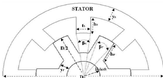
Figure 1. Cross section of 8/6 SRM in unaligned position
