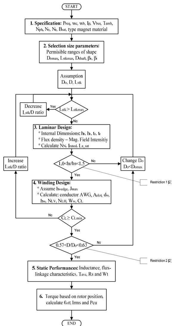
Figure 2. Flow chart of the CAD Program SRM
