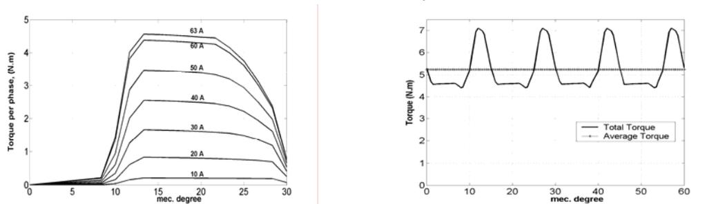
Figure 6. a) Torque vs. rotor position characteristic for SRM CAD-design. b) Total developed torque.
