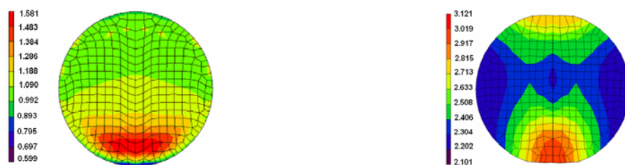
(a) Cross section after the 1 st ECAE extrusion (b) Cross section after the 2 nd ECAE extrusion Figure 3. Strain field in the work-piece processed by ECAE using route A
