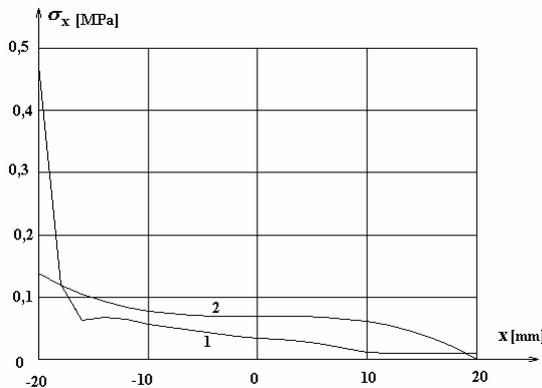
Figure 8. Diagrams of the variation of normal stresses  $\sigma_x$  for the local area  $y=-b$  in  $x \in [-c, c]$
