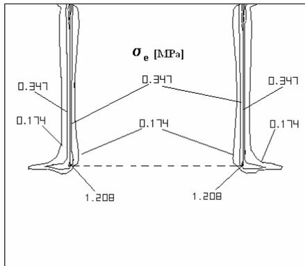
Figure 2 Equivalent stresses of Tresca in the inferior universal iron
