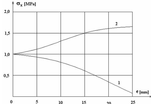
Figure 9. Variation diagrams of the stresses  $\sigma_x$  in the inferior universal iron for the case in which eccentricity “e” is variable
