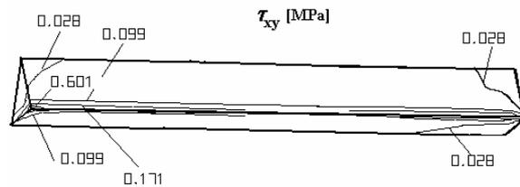
Figure 5. Tangential stresses vary, in the dangerous sections
