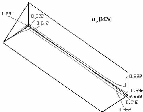
Figure 4 Equivalent stresses of Tresca in the cordon welding
