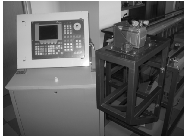
Figure 4. Computer Numerical Control and drive unit
