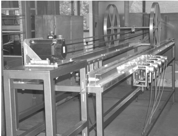
Figure 3. Rail of measure stand with assembled measuring units
