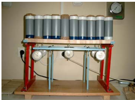
Figure 8. The experimental device used to measure the deflection in the five points indicated in figure 8.
