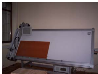
Figure 4. CADesQ equipment used to measure the panels flatness.
