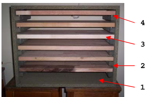
Figure 3. The device in which the panels were supported on; 1-rack; 2-wooden fillet; 3-panel; 4-fulcrums.
