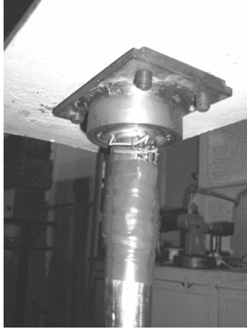
Figure. 2. The mixer shaft with electro resistive traductors
