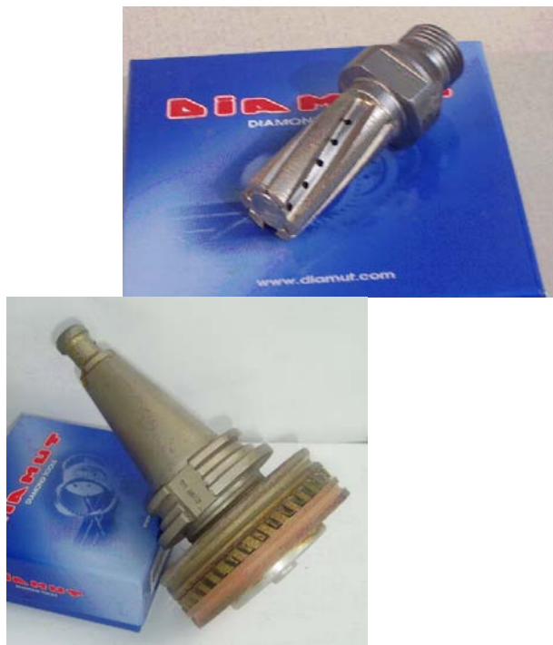
Figure 1. A diamond cutter and a combined tool for glass edge machining.
