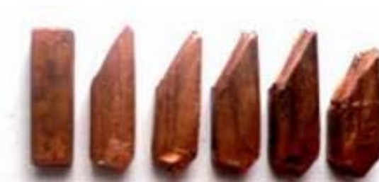
Figure 2. Copper samples after individual passes with using the ECAP technology
