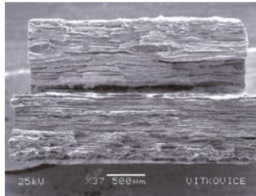
Figure 4. Lamellar structure of low carbon steel after deformation e = 8,8
