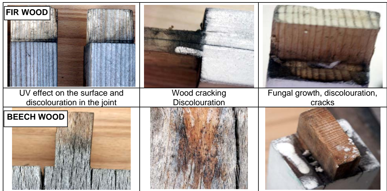
Figure 2 Examples of degradation phenomena observed after 27 months exposure
