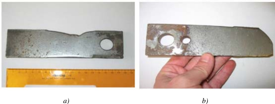
Figure 2. Worn thresher knives with injected protective coating; a) fixed; b) rotating
