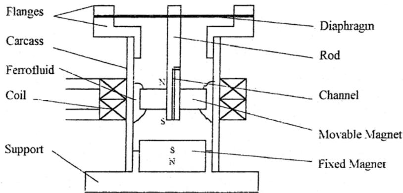
Figure 1. schematic diagram of electromechanical convertor.
