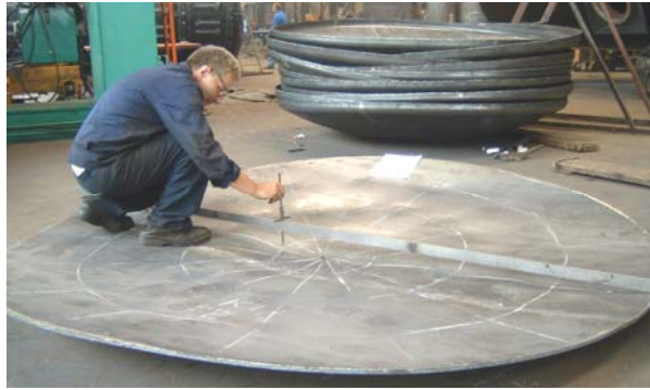
Figure 4. Measurement of buckled plate geometry.
