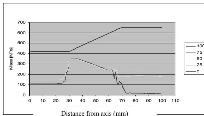
Figure 6. Distribution of the von Mises equivalent stress in the case of conical parts made by using a cylindrical punch for different blankholder forces
