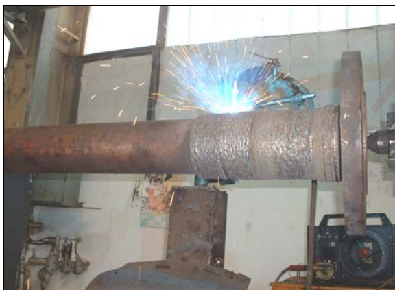
Figure 3. The surfacing layer of an axes part as well as the leading-belt \Phi 630 \times 1400 after surfacing.
