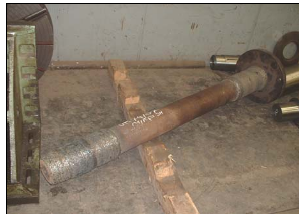
Figure 3. The surfacing layer of an axes part as well as the leading-belt \Phi 630 \times 1400 after surfacing.
