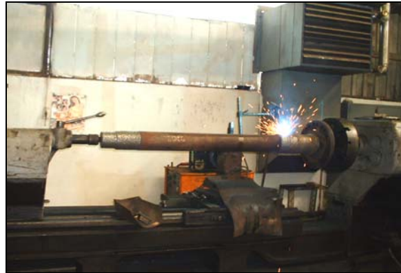
Figure 2. Surfacing process of the axis.
