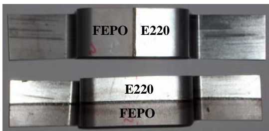
Figure 6. Parts made by TWBs with transversal and longitudinal weld line
