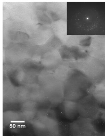
Figure 2. Bright field transmission electron micrograph of  $Nd_{14}Fe_{79}B_7$  alloy in optimized magnetic state. The insert figure is the electron diffraction pattern of the selected area.
