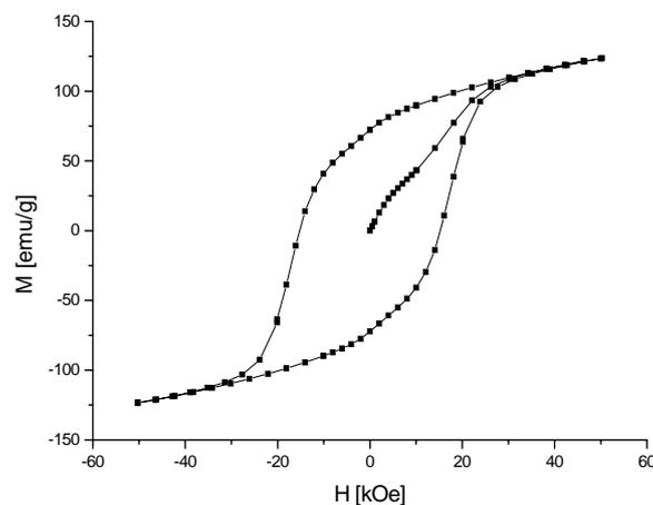
Figure 3. SQUID hysteresis loop of  $Nd_{14}Fe_{79}B_7$  alloy in optimized magnetic state
