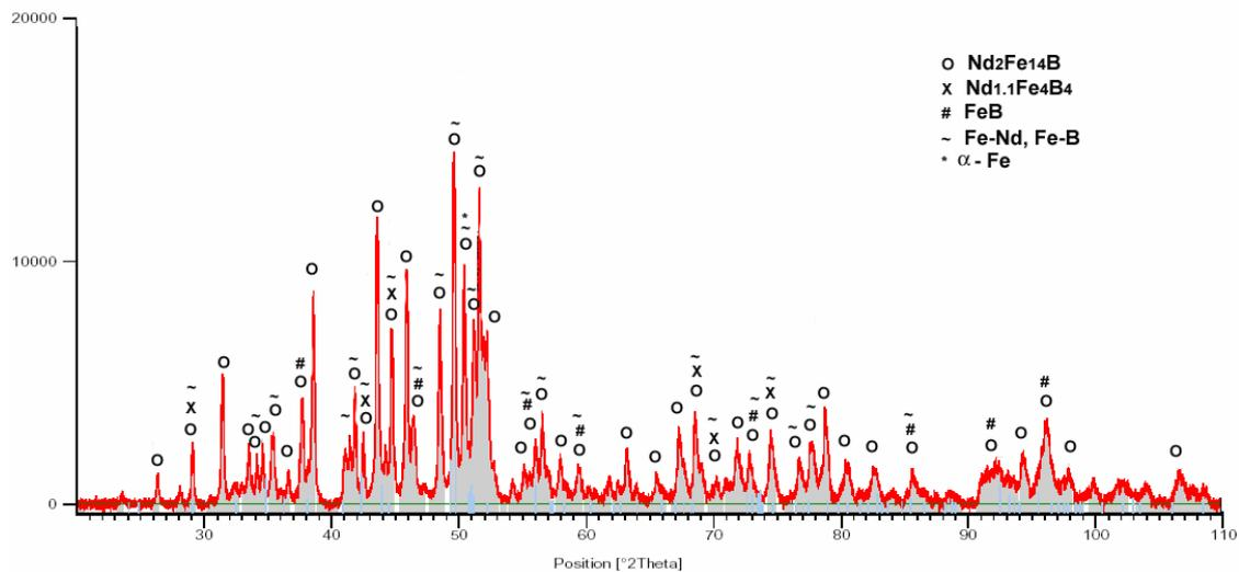
*Figure 1. The X-ray diffractograms of Nd<sub>14</sub>Fe<sub>79</sub>B<sub>7</sub> powder in optimized magnetic state*
