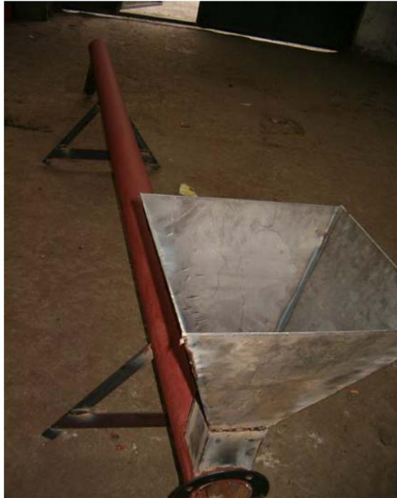
*Figure 2. Experimental installation for adding covering and thermoinsulating powder in tundish*
