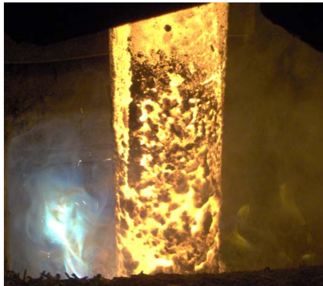
Figure 3. Mode of adding the micro-coolants in the mould of the continuous casting machine.
