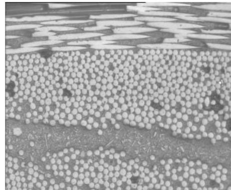
*Figure 2. Cross-sectional optical micrograph illustrating laminated construction typical of continuous fibre composite materials (glass-fibre epoxy fabric). 100x*
