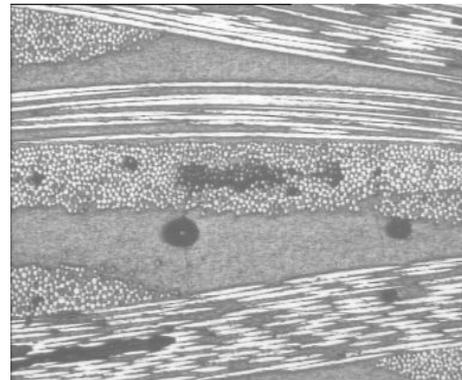
*Figure 4. Microstructure of Kevlar - vinylester fabric with debonds. 50x*
