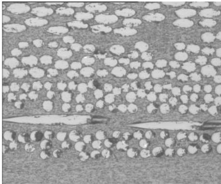
*Figure 1. Microstructure of Kevlar - vinylester fabric. 200x*
