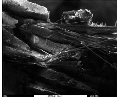
Figure 6. Typical fracture pattern of fatigue of laminates. 32x
