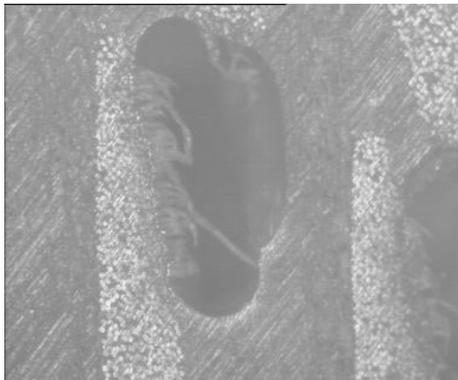
*Figure 3. Microstructure of Kevlar - epoxy fabric with debond. 50x*
