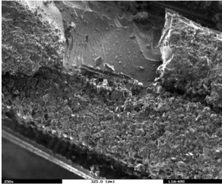
Figure 5. SEM micrograph of broken epoxy resin. 250x
