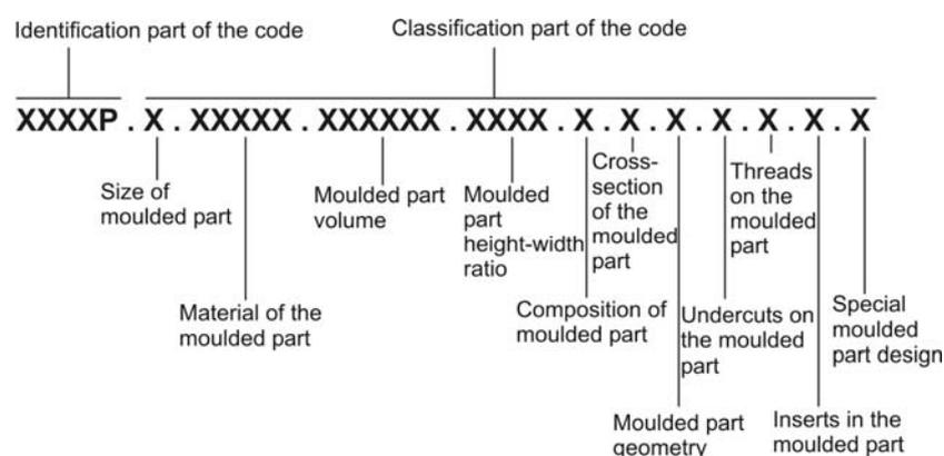
Figure 2. Classification code of the moulded part
