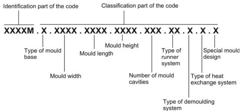
Figure 3. Mould classification code
