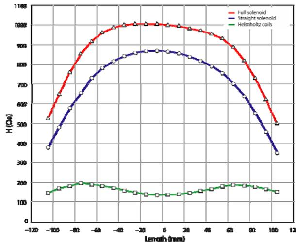
Figure 2. Experimental characterization of the solenoid with MG-4D Gaussmeter (Walker Scientific)
