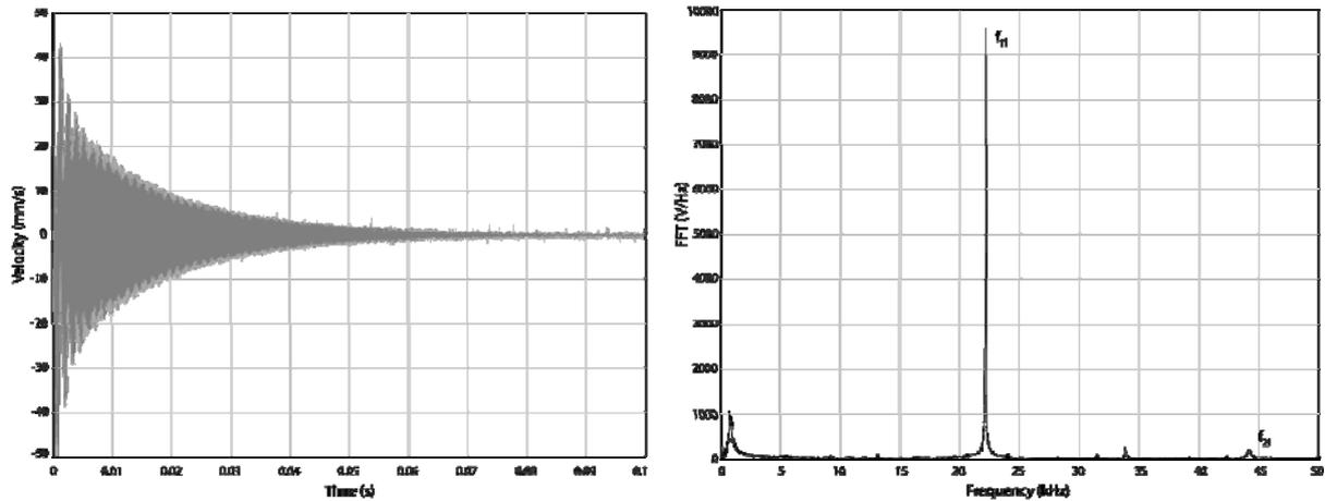
Figure 3. Temporal response (left) and FFT (right) of an unmagnetized nickel rod
