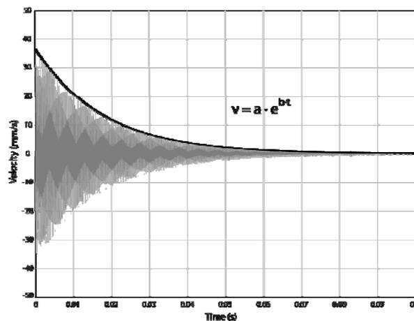
Figure 4. Exponential envelope for an acquired signal
