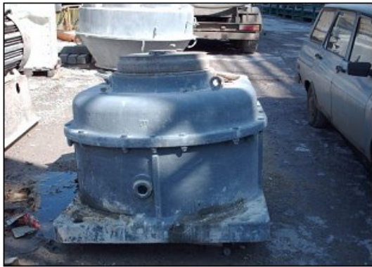
Figure 2. Cracked gearbox frame around its base
