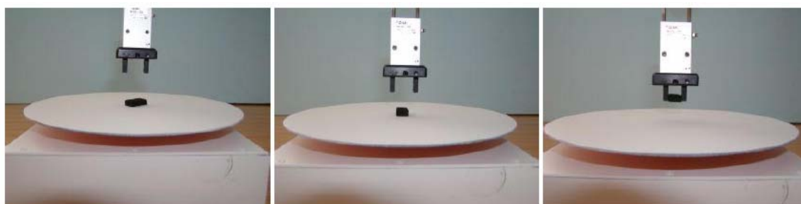
Figure 6. Example of part non-collision positioning for manipulator gripping with pneumatic effector
