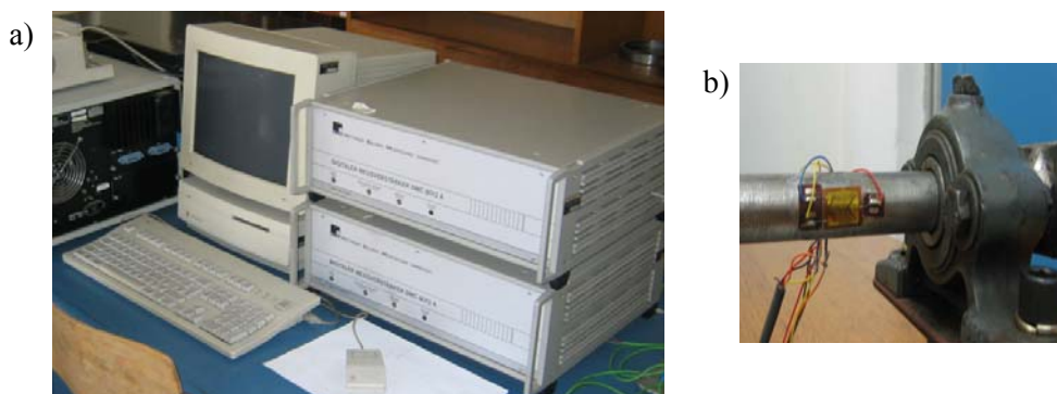
Figure 1. HBM digital measuring amplifier DMC 9012A and analised measuring spot of modele device for torsion
