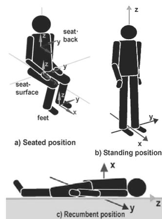
Fig. 1. Coordinate system to evaluate whole-body vibration (from ISO 2631)
