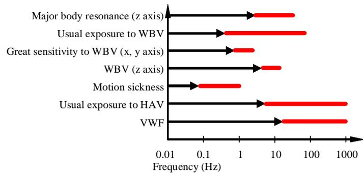
Fig. 4. Frequency-dependent effects of vibration on human body
