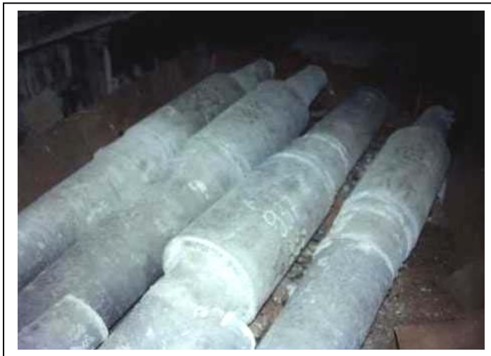
Figure 6. Rough-cast rolls for rolling.
