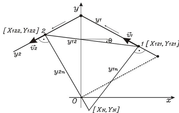
Figure 6. Velocity and instantaneous pole of velocity
