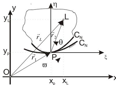
Figure 4. Kinematic of centrodes curvature
