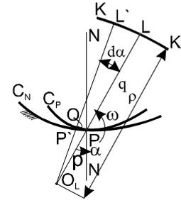
Figure 5. Position and radius of roulette k-k
