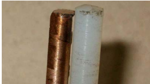
Figure 6. Comparison between bronze and Ertalon66SA test specimen
