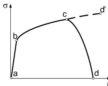
Figure 1. Uniaxial stress-strain response of a metal specimen.
