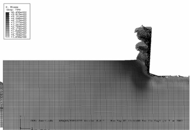
Figure 3. Von Mises stress with applying material damage effects.
