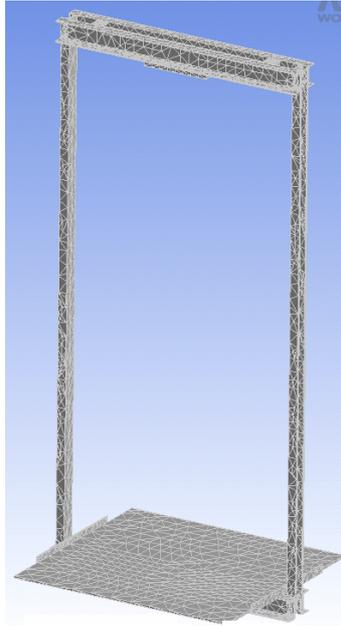
Figure 2. Isometric view of the car sling model
