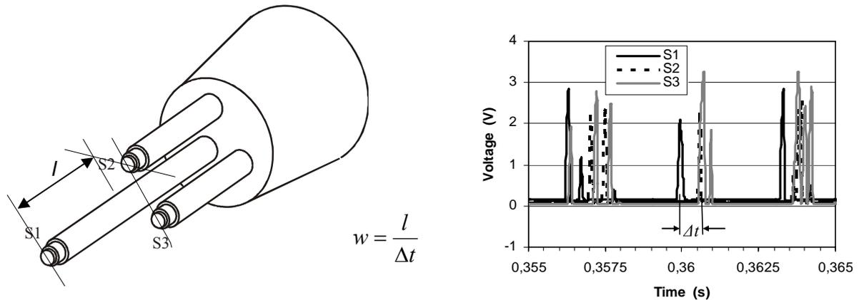
Figure 4: Shot velocity measurement
