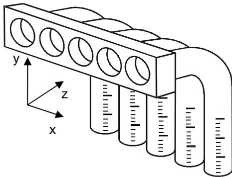
Figure 2: Multi hole collector
