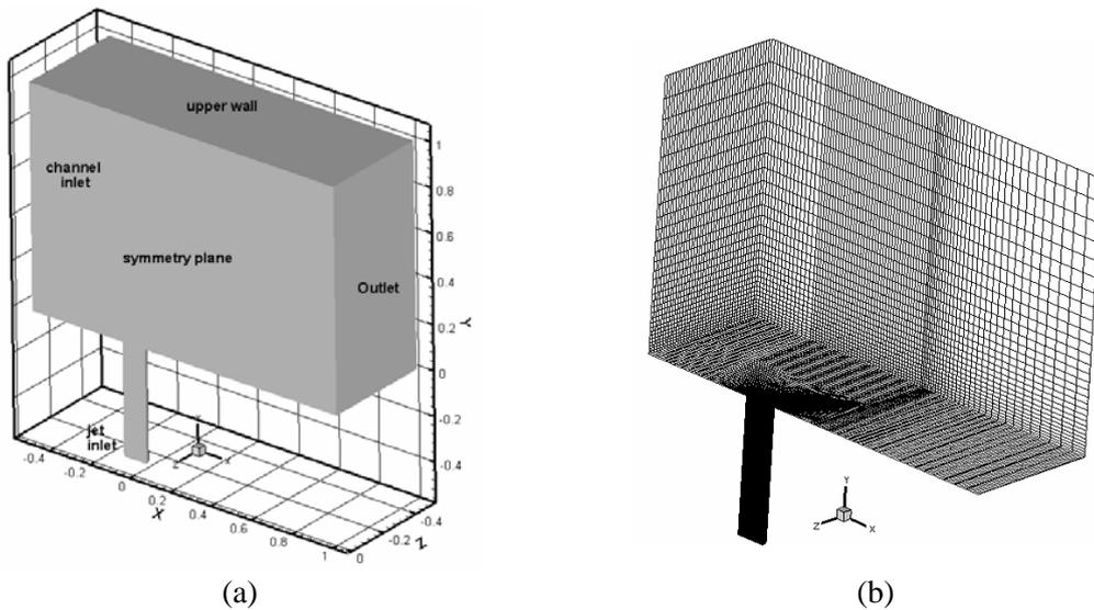
Figure 2. *Working domain and coordinate system (a), grid structure (b).*
