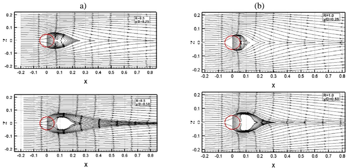
Figure 4. CVP evolution at different normal stations for a)  $R=0.5$  and b)  $R=1.0$ .
