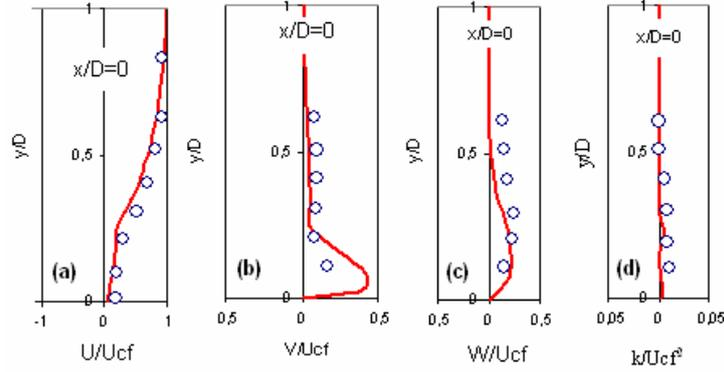
Figure 1. *U-velocity (a), V-velocity (b) and W-velocity (c) comparisons of RSTM data with experimental results of Ref. [8] for  $z/D=0$ ,  $R=0.5$ , Circle: exp., solid: CFD.*
